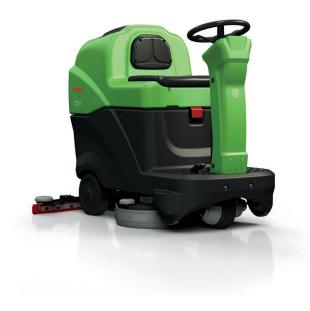
The **CT 80** is the smallest ride-on scrubber dryer in our range, but is still designed on a robust industrial platform. There are 2 different types, one for highly professional two-brush applications (CT80-BT55 ECO) and another for less intensive single brush uses (CT80-BT70). Though extremely compact (length only 130 cm), the CT 80 nevertheless carries an 83 litre solution tank that gives better than average autonomy for this class of machine.
