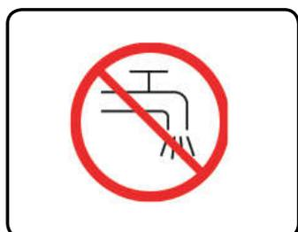
NE PAS ALIMENTER AVEC DE L'EAU POTABLE. UTILISER UN DISCONNECTEUR CONFORMÉMENT À LA NORME EN 12729 TYPE BA.
